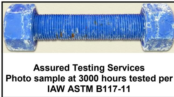
SoCote™3D offers excellent corrosion resistance of up to 3,000 Salt Spray Hours. The samples provided to Assured Testing Services were tested per IAW ASTM B117-11 and showed less than 15% red rust after 3,000 Salt Spray Hours.
